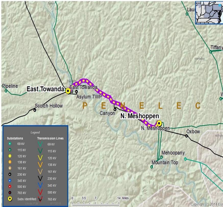
The recommended solution – Baseline Project b3137, rebuilds 20 miles of the East Towanda - North Meshoppen 115 kV line and adjusts relay settings at East Towanda and North Meshoppen 115 kV substations (new rating 202N/245E summer 228N/290E winter). The recommended solution addresses the baseline needs in the area. The estimated cost for this project is \$58.6 million, and the projected in-service date is June 2024. The local transmission owner, Penelec, will be designated to complete this work.
