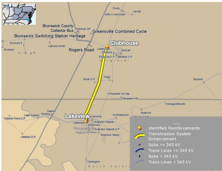
The recommended solution is to rebuild the Clubhouse-Lakeview 230 kV line with single circuit wood pole equivalent structures at the current 230 kV standard, with a minimum rating of 1047 MVA (Existing Rating = 399 MVA). The estimated cost for this project is \$27 million, and the projected in-service date is December 2024. The local transmission owner, Dominion, will be designated to complete this work.
