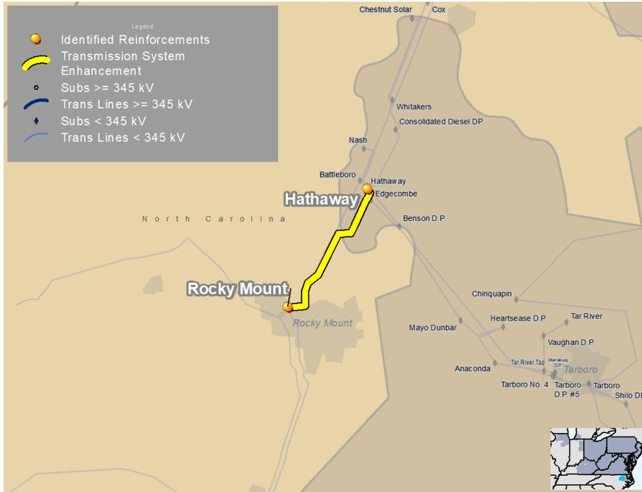
The recommended solution is to rebuild Hathaway-Rocky Mount (Duke Energy Progress) and Hathaway-Nash-Rocky Mount 230 kV lines with double circuit steel structures, using double circuit conductor at current 230 kV standards, with a minimum rating of 1047 MVA (Existing Rating = 478 MVA). The estimated cost for this project is \$13 million, and the projected in-service date is December 2024. The local transmission owner, Dominion, will be designated to complete this work.
