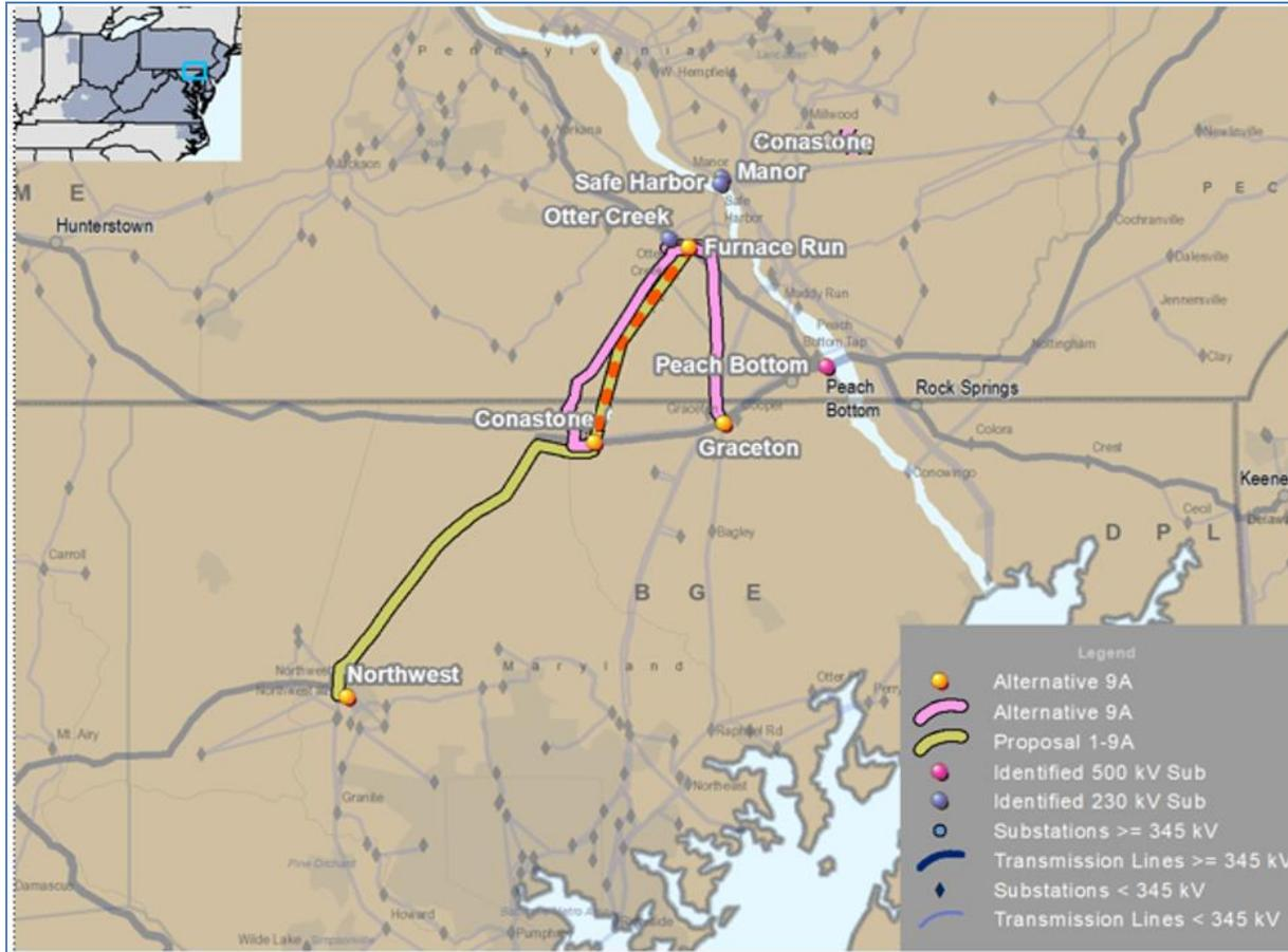
\* Note: Dotted red line depicts originally proposed Furnace Run-Conastone 230 kV line now being rerouted
