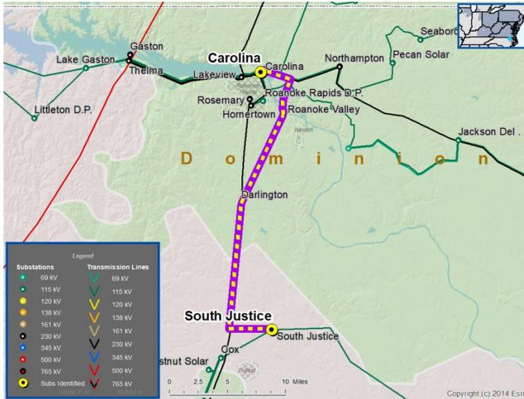
The recommended solution is to rebuild the 18.6 mile section of Carolina – South Justice Branch 115 kV which includes 1.7 miles of double circuits. This segment of Carolina – South Justice Branch 115 kV will be rebuilt to current standards with a minimum rating of 261 MVA. The secondary circuit rating will not change. The estimated cost for this project is \$25 million, and the projected in-service date is December, 2025. Dominion will be designated to complete this work.
