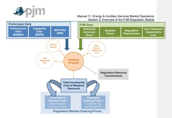
MCE ranks all available regulating resources in ascending merit order price, and simultaneously determines the least expensive set of resources necessary to provide energy, regulation and synchronized reserve for the operating hour taking into account any resources self-scheduled to provide any of these services. The Rank price is determined as follows:
