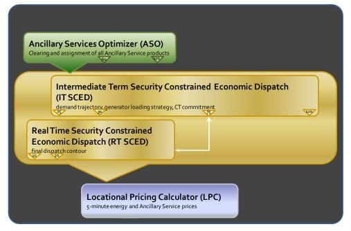
The applications jointly optimize the products on a 5-minute basis to ensure that all system requirements are met using the least cost resource set.
