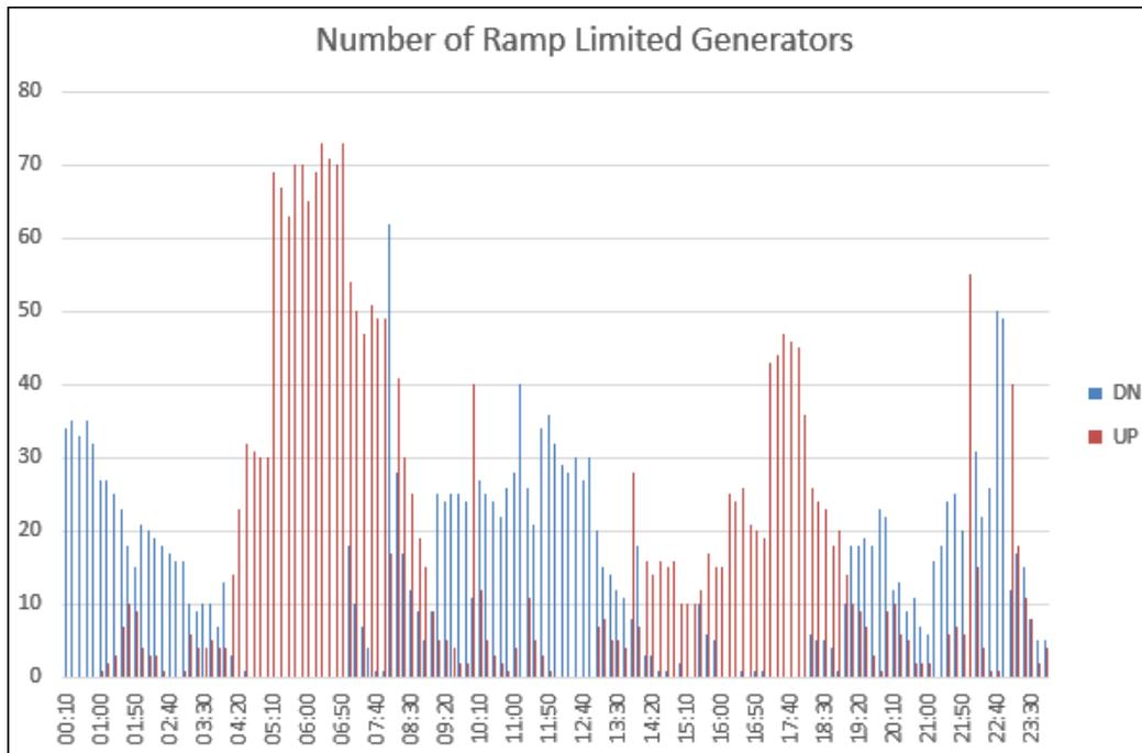
Figure 2-22: Number of Ramp-constrained Units per 10-minute Interval (20% HOB0, January 8)
