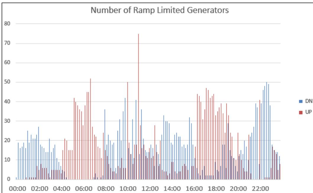
Figure 2-18: Number of Ramp-constrained Units per 10-minute Interval (20% HSBO, March 4)
