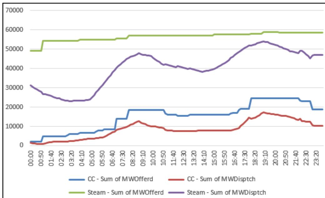
Figure 2-47: Thermal Generation MW Offered vs. Dispatched, On-line Units Only (30% HOBO, January 12)
