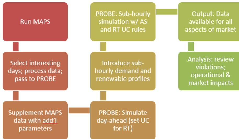
**Figure 2-1: GE MAPS-to-PROBE Simulation Process**
