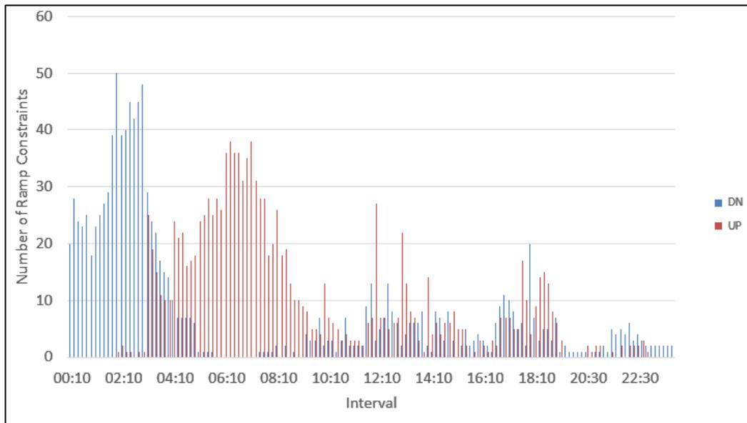
Figure 2-3: Number of Ramp-constrained Units per 10-minute Interval (2% BAU, July 15)
