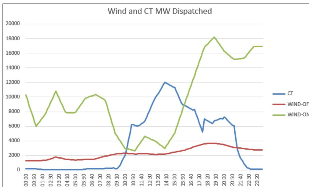
Figure 2-32: Wind vs. CT Dispatch for Each Interval
