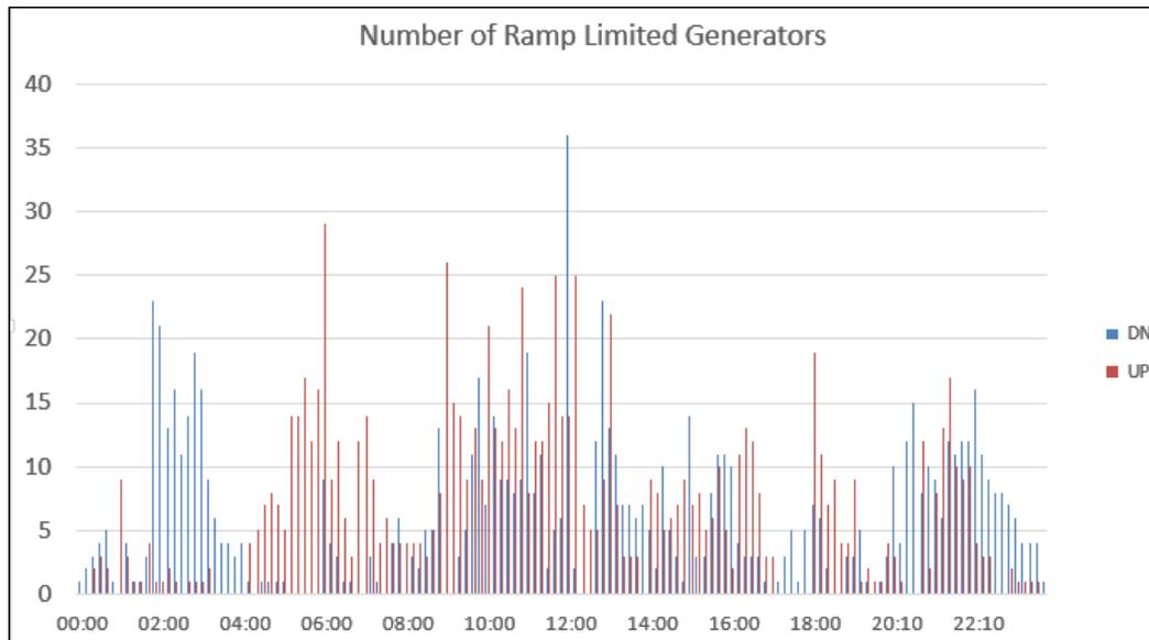
**Figure 2-8: Number of Ramp-constrained Units per 10-minute Interval (2% BAU, July 28)**
