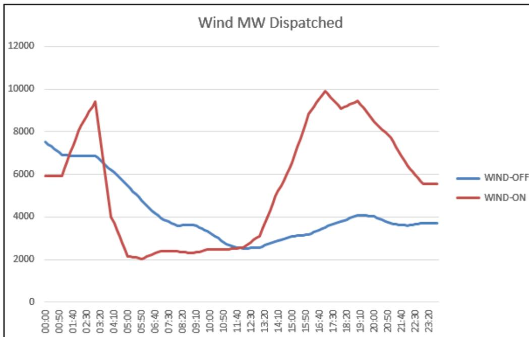
Figure 2-23: Wind Dispatch for Each Interval (20% HOBO, May 26)
