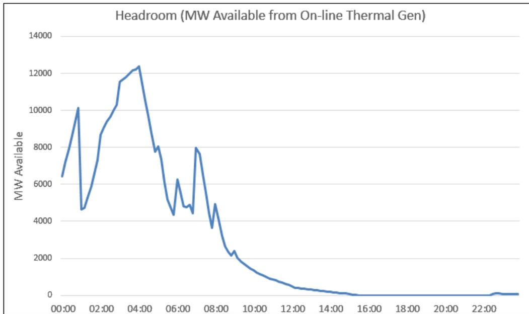
**Figure 2-15: Headroom - MW Available from Thermal Generation (14% RPS, August 3)**
