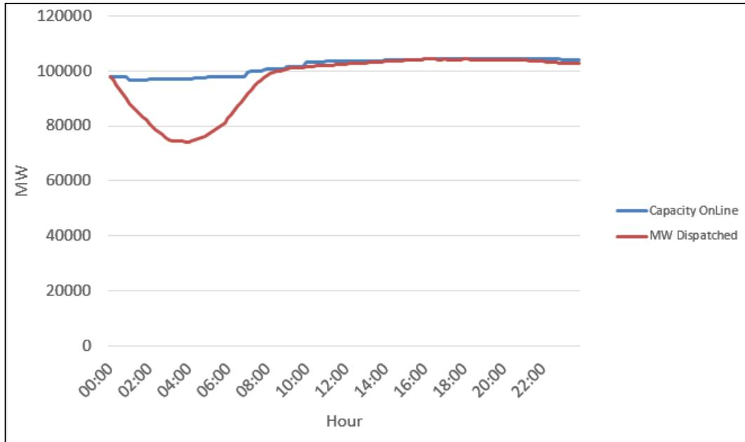
Figure 2-2: On-line Capacity vs. MW Dispatched for Steam + Combined Cycle (2% BAU, July 15)
