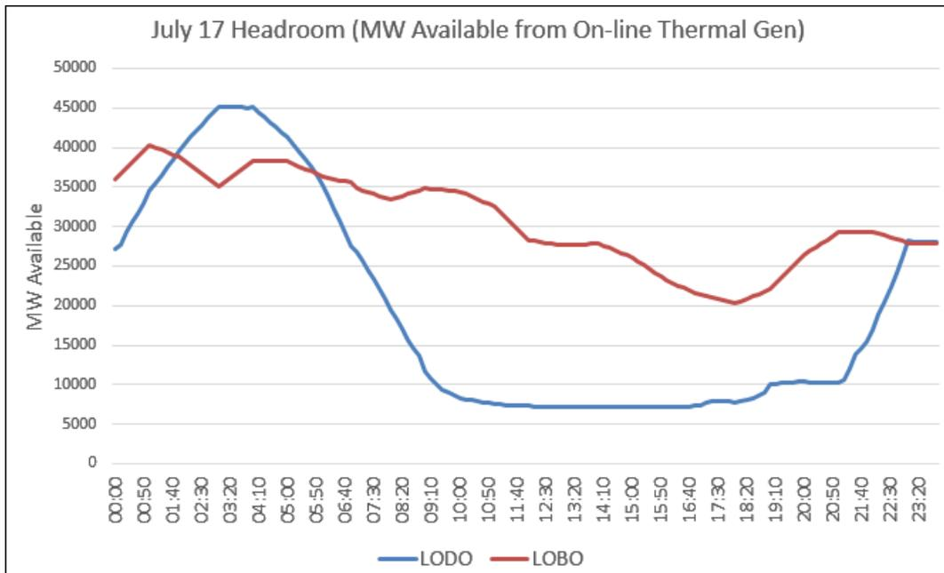
Figure 2-38: Headroom - MW Available from Thermal Generation (20% LODO, July 17)
