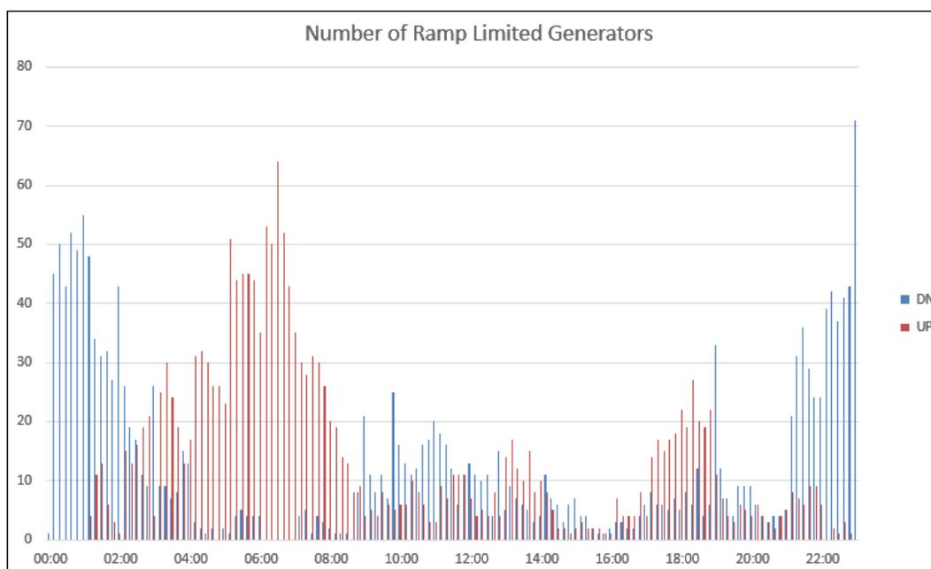
Figure 2-10: Number of Ramp-constrained Units per 10-minute Interval (14% RPS, February 12)
