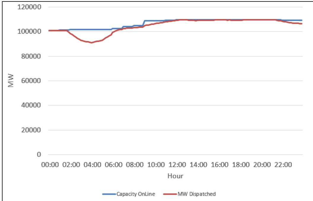
**Figure 2-6: On-line Capacity vs. MW Dispatched for Steam + Combined Cycle (2% BAU, July 28)**
