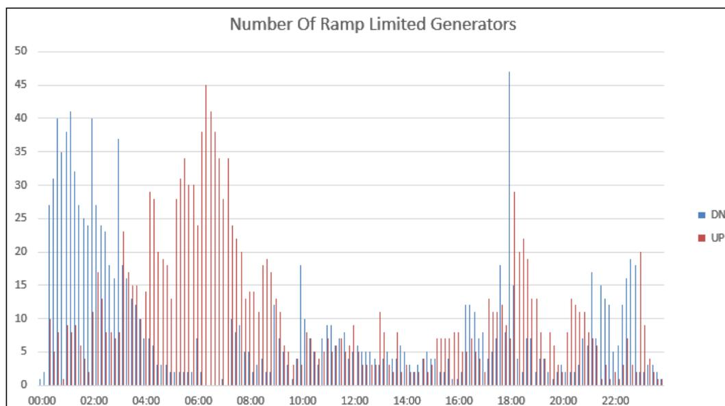
Figure 2-11: Number of Ramp-constrained Units per 10-minute Interval (14% RPS, March 2)
