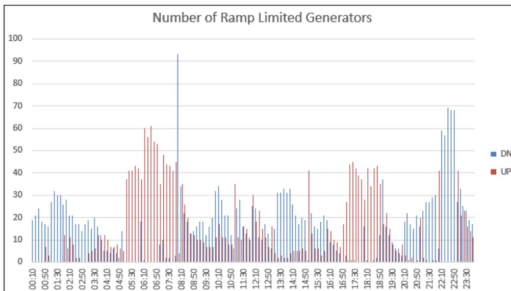
Figure 2-33: Number of Ramp-constrained Units per 10-minute Interval (20% LODO, March 4)
