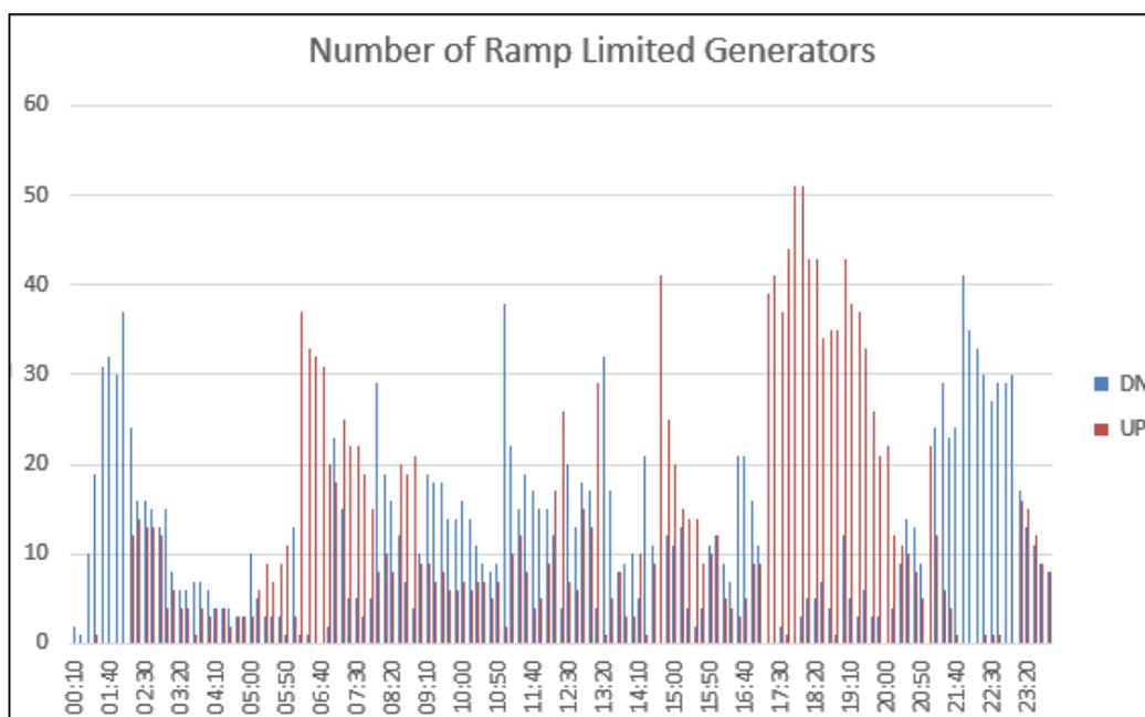
**Figure 2-43: Number of Ramp-constrained Units per 10-minute Interval (30% HSBO, April 12)**
