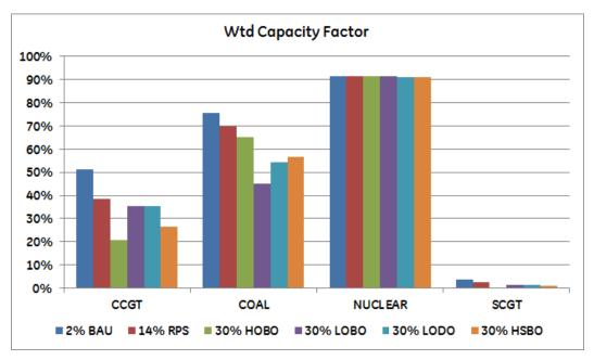
Figure 1-15: Capacity Factor by Unit Type (30% Scenarios)
