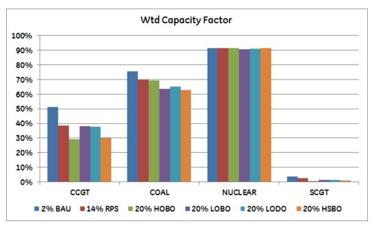
Figure 1-14: Capacity Factor by Unit Type (20% Scenarios)
