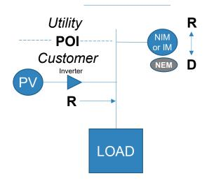
NIM – Non-Interval Meter IM – Smart Meter NMP – Non-PJM Market Participant Facility BM – Bi-directional Meter PV – Photovoltaic NEM – Net Energy Meter Rider
