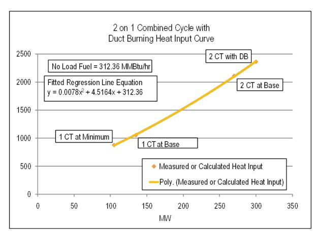
Each diamond in the graph above is a design heat input data point obtained from the original equipment manufacturer or calculated by heat balance. A regression analysis was performed on the design data to obtain the unit's Heat Input curve as a function of unit output levels with natural gas as a fuel:
