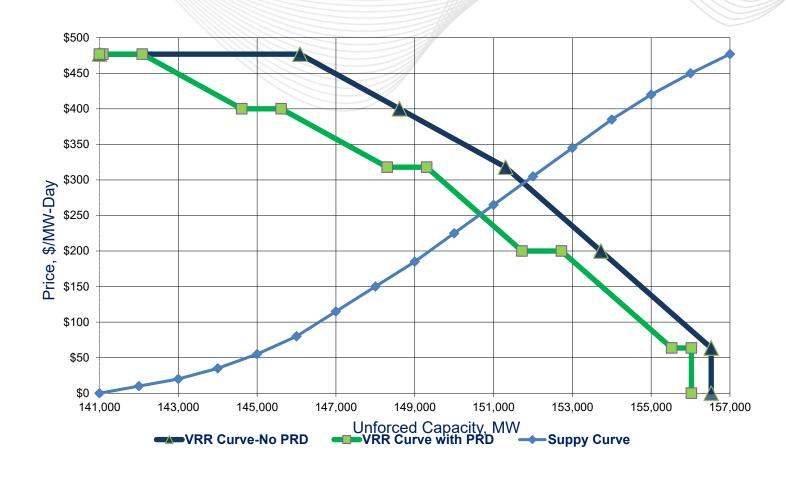
PRD will shift the demand curve to the left which will reduce the overall capacity requirement
