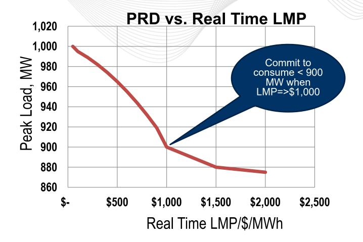
Load that will automatically respond to energy prices and be off the grid during a PJM emergency (PAI) and therefore the LSE will receive a lower capacity requirement.
