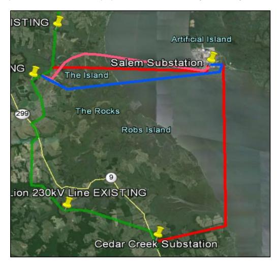
Salem substation is located on the New Jersey side of the Delaware River; the 230kV Red Lion transmission line is located going north to south on the Delaware side of the Delaware River.
