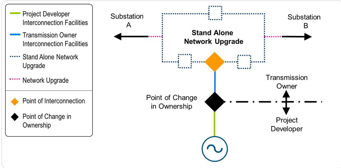
Exhibit 10: Generator Interconnection into Existing TO Substation
